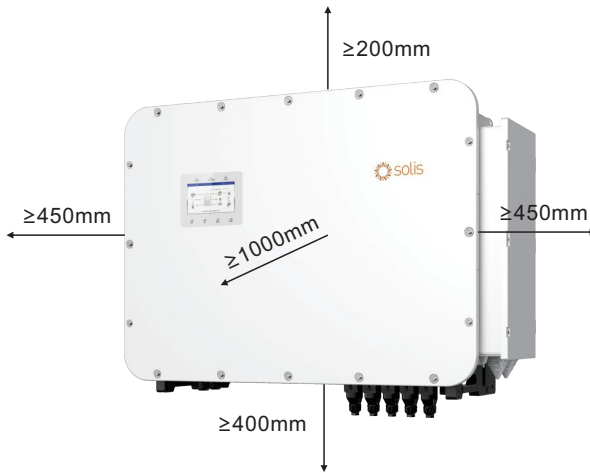
Figure 3.3 Inverter Mounting Clearances
